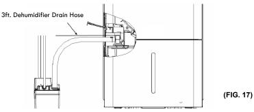
**NOTE:** If you need to cut the dehumidifier drain hose, only cut on the flat end of the hose. Do not cut the angled end as it is designed for insertion into the pump.
